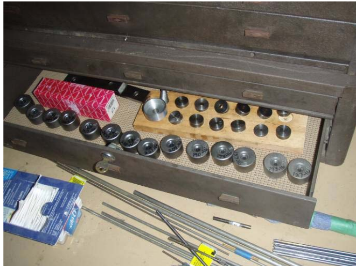
Fig 10 – Carbide Die Set with Mandrels
