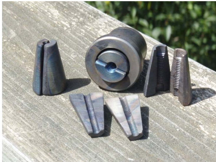
Fig 6 – Split Cone Jaw Set with Holder
