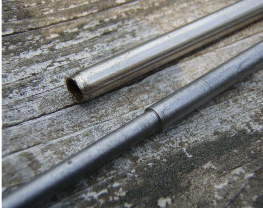
Fig 5 – Rolled NS Tube and Step-Down Mandrel
