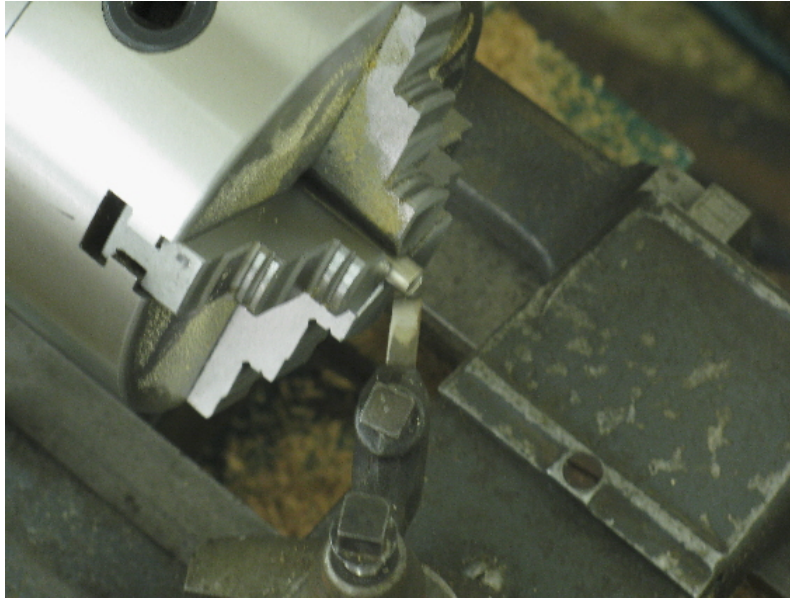
Fig 4 – Rolling over the NS Tube end in a lathe
