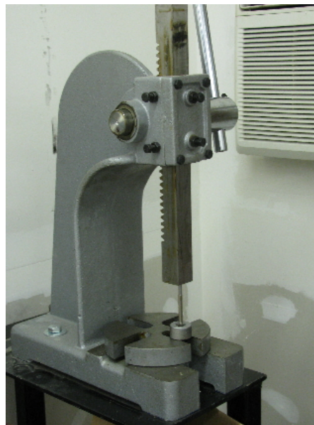
Fig 9 – Arbor Press for Pushing Tubing
