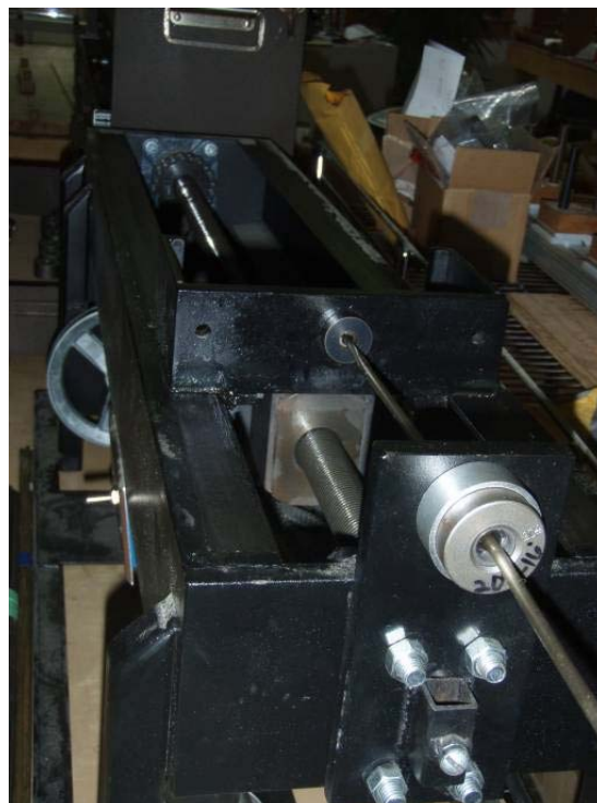
Fig 11 – Drawing NS Tube through a Carbide Die
